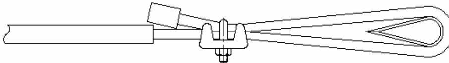
Center the thimble in the loop, and apply the second clip as close to the thimble as possible. Try to keep cable lengths as straight and even as possible. Tighten nuts evenly, alternating from one to the other, until reaching the specified torque.
